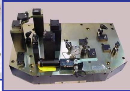
Power workholding fixtures are an effective way to increase productivity, enhance quality, reduce labor and minimize part-to-part changeover times.
